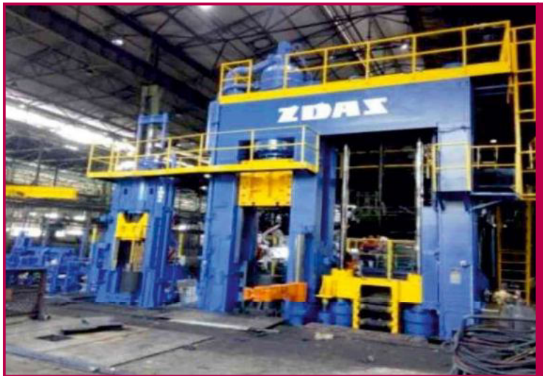
ROBOTIC FORGING PLANT FOR HIGH CALIBER SHELL
